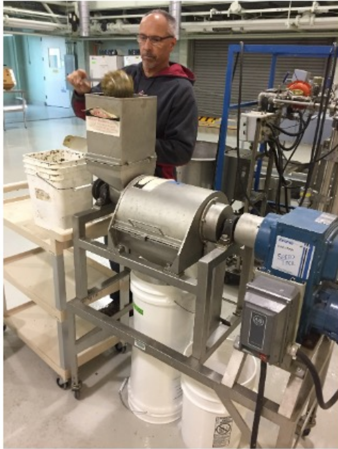
Finisher for olive Pomace pit separation
