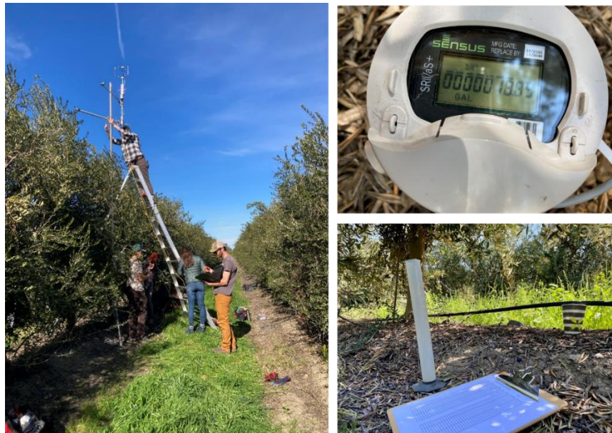
Fig 1 - ET tower installation (left), flow meter and distribution uniformity measurements (right)
