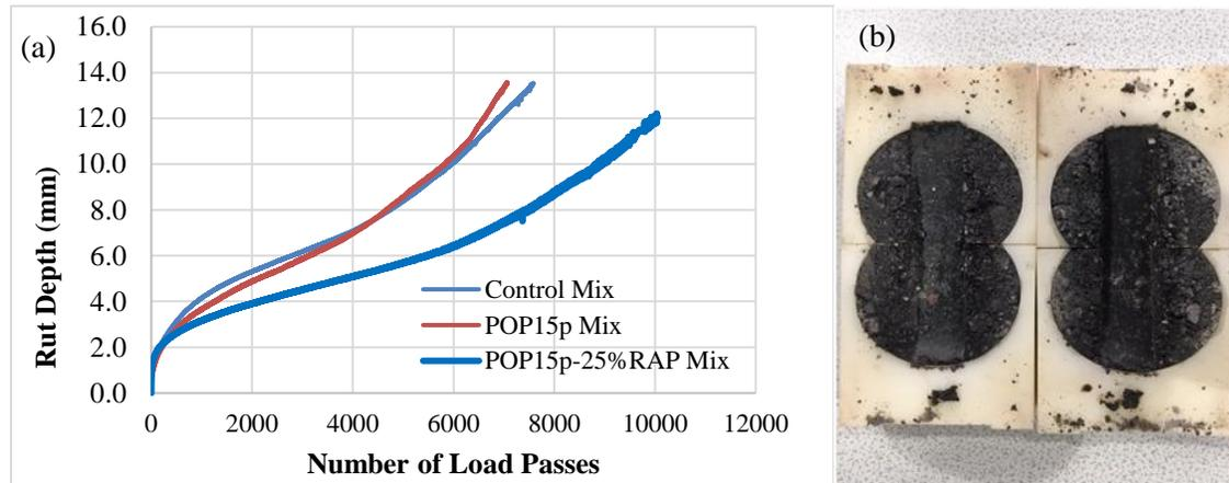
**Figure 18. (a) HWTT results and (b) evidence of moisture stripping for the control mixture.**
