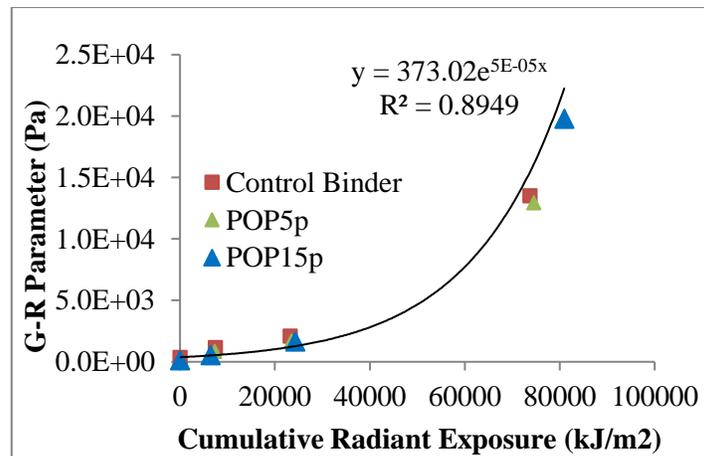
**Figure 9. Changes of G-R parameters with cumulative radiant exposure.**
