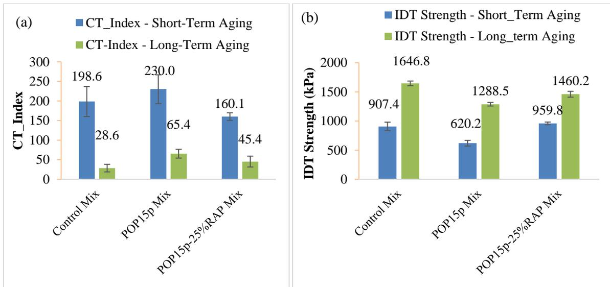
**Figure 17. (a) Cracking tolerance index ( $CT_{index}$ ) and (b) IDT strength of mixes after short-term aging (60°C for 16 hours and 145°C for 2 hours on loose mixes) and long-term aging (145°C for 2 hours, 85°C for 120 hours, and 145°C for 2 hours on loose mixes).**
