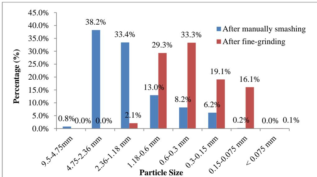
**Figure 1. Coffee grinder used to process olive pomace and particle size distribution of olive pomace after manually smashing and after fine-grinding using the coffee grinder.**
