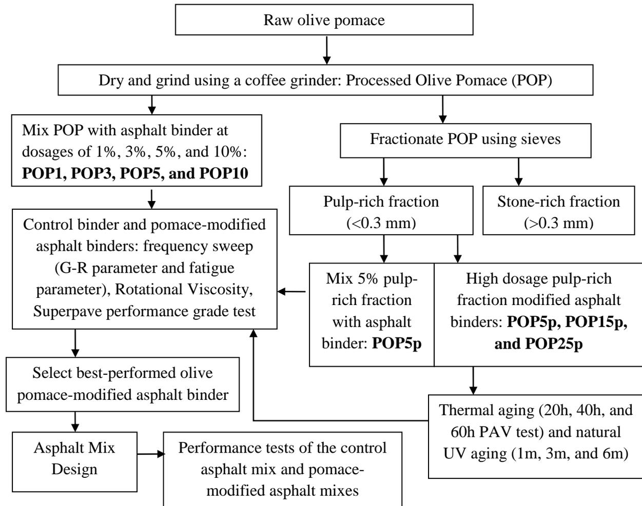
**Figure 2. Flow chart of the testing plan.**
