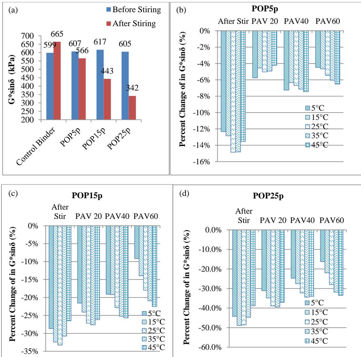
**Figure 11. (a) Fatigue parameters ( $G^* \cdot \sin \delta$ ) at 25°C before and after 85-minute stirring and percent changes in  $G^* \cdot \sin \delta$  for (b) POP5p, (c) POP15p, and (d) POP25p binders compared with the control binder after 85-minute stirring and long-term PAV aging.**
