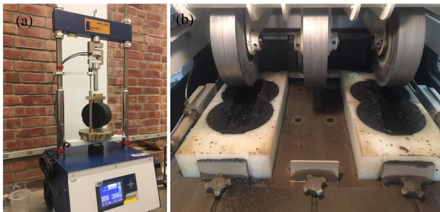
**Figure 6. (a) Test set-up of indirect tensile (IDT) strength for moisture and cracking resistances and (b) Hamburg wheel tracking test for rutting resistance.**
