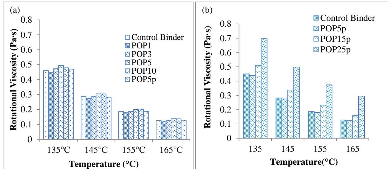
**Figure 12. Rotational viscosity results of (a) pomace modified asphalt binders and (b) high dosage pulp-rich fraction modified asphalt binders after 85-minutes stirring.**
