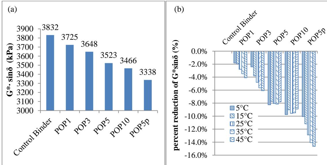
**Figure 10. (a) parameter ( $G^* \cdot \sin \delta$ ) results at 25°C and (b) percent reduction of fatigue parameter of pomace-modified asphalt binders.**
