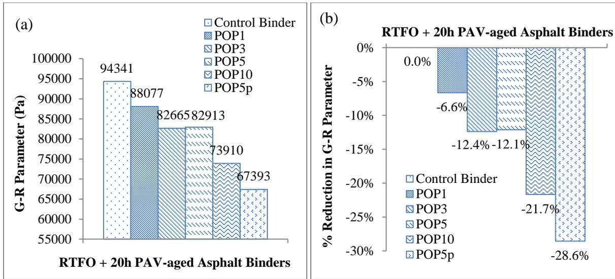
**Figure 7. (a) G-R parameter and (b) percent reduction in G-R parameter of the control and POP-modified asphalt binders.**
