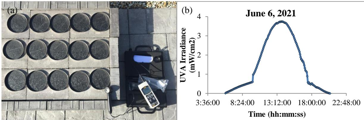
**Figure 3. (a) Asphalt samples of the control binder, POP5p, and POP15p conditioned outdoor and (b) a typical daily UVA irradiance at 365nm wavelength using a UV meter.**
