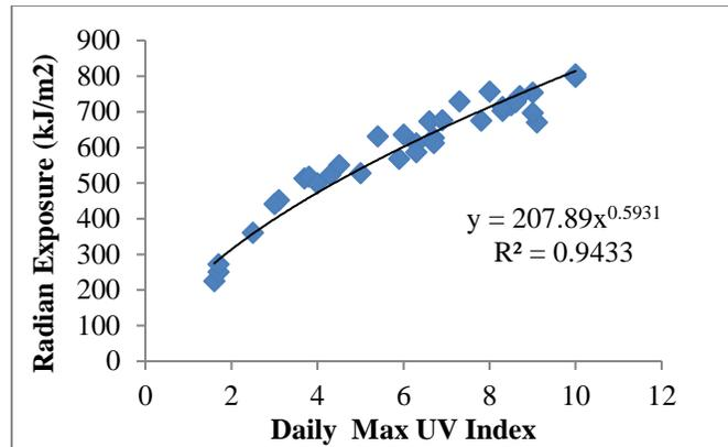
**Figure 5. Regression between daily maximum UV index and measured radiant exposure at UVA wavelength of 365nm.**
