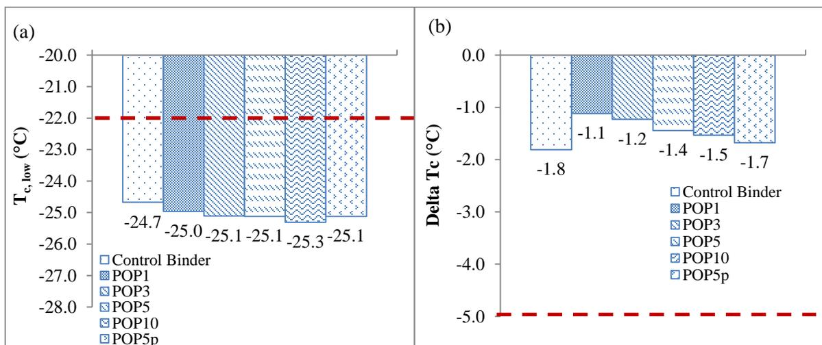
**Figure 15. (a) Critical low failure temperature ( $T_{c,low}$ ) and (b)  $\Delta T_c$  results of the control binder and pomace-modified asphalt binders.**
