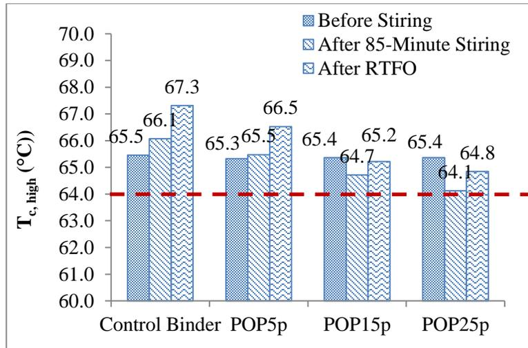
**Figure 14. Critical high failure temperature ( $T_{c,high}$ ) of high dosages of pulp-rich fraction modified asphalt binders before and after 85-minute stirring and after RTFO aging.**
