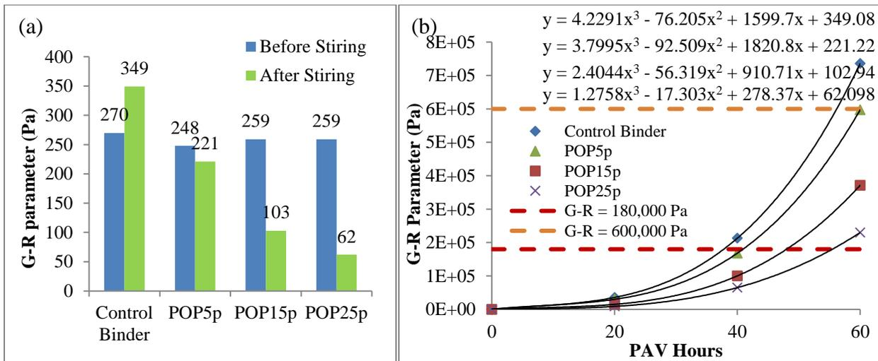
**Figure 8. (a) G-R parameters before and after 85-minute stirring at 160°C and (b) G-R parameters after the long-term PAV aging (20h, 40h, and 60h).**
