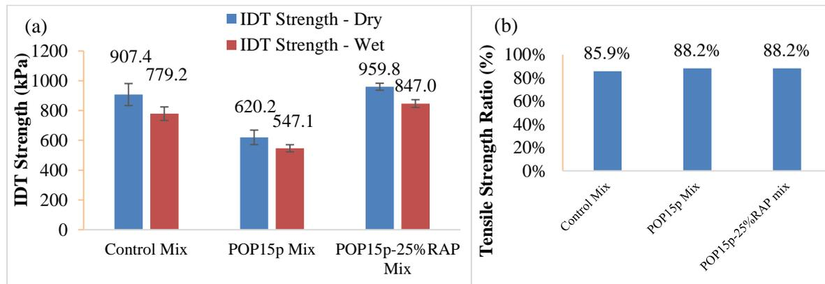
**Figure 16. Results of (a) dry and wet IDT strength and (b) tensile strength ratio of mixes.**
