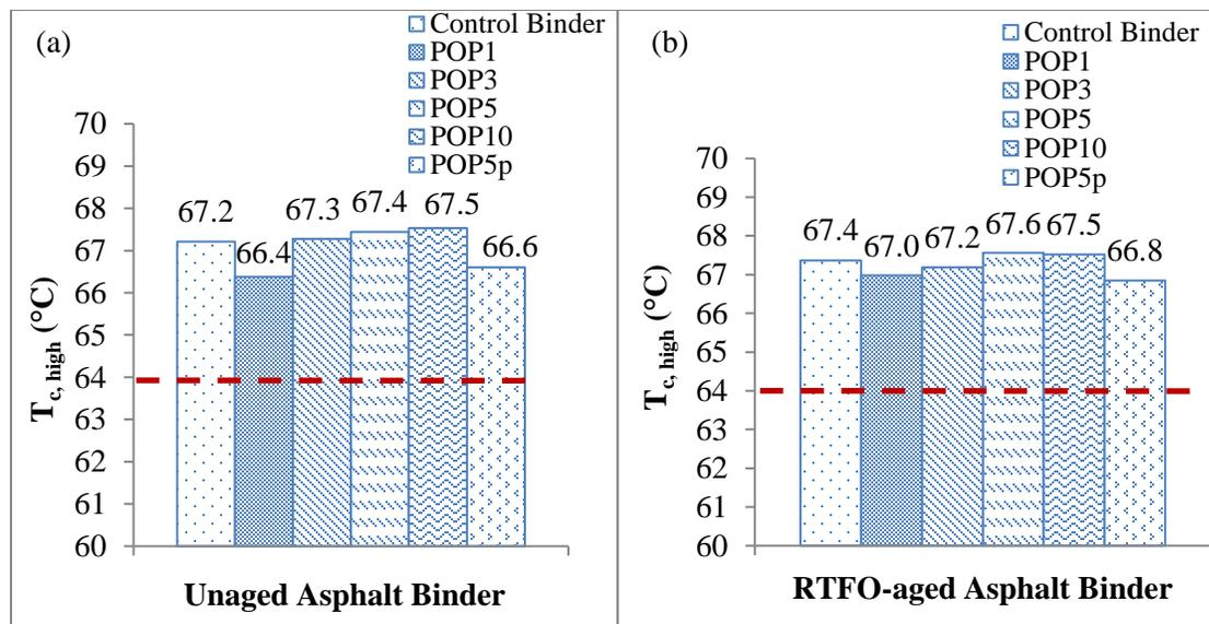
**Figure 13. Critical high failure temperature ( $T_{c, high}$ ) of unaged and RTFO-aged asphalt binders.**
